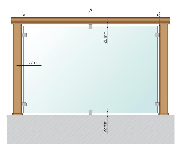
A - If the glass has a wider dimension than 1400 mm, extra clamps will be needed at the top and bottom to support the glass. For dimensions over 1700 mm, we recommend a total of four glass clamps for the upper and lower edges. 'A' denotes the width of the opening and also the dimensions to be specified in the configurator.
