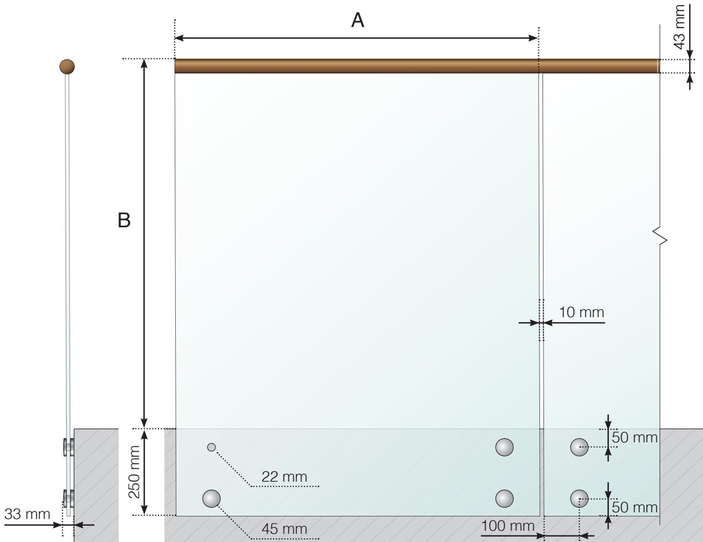
A - The width of the glass depends on the length of the sides and the number of sections
