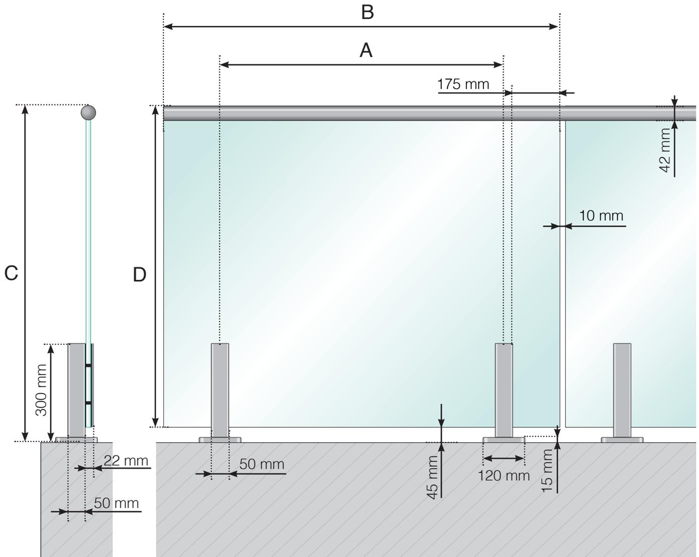
A - The c/c dimensions of the posts depend on the length of the sides and the number of sections
