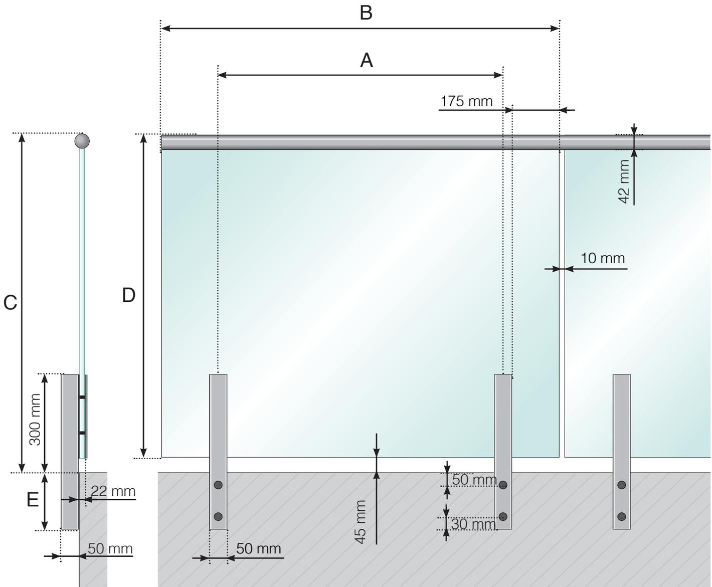
A - The c/c dimensions of the posts depend on the length of the sides and the number of sections
