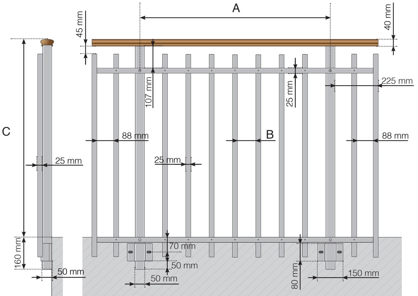
A - The c/c dimensions of the posts depend on the length of the sides and the number of sections
